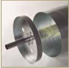
12" diameter drums allow for lower headroom requirements. An enclosed barrel houses the dead axle assembly and protects the factory lubricated springs from direct contact with environmental elements. The inherent strength provided by the spiral barrel minimizes axle deflection providing smoother operation. Because the curtain is attached by screws and not seamed to the barrel, replacement of either independent assembly is cost-effective, quick and easy.
